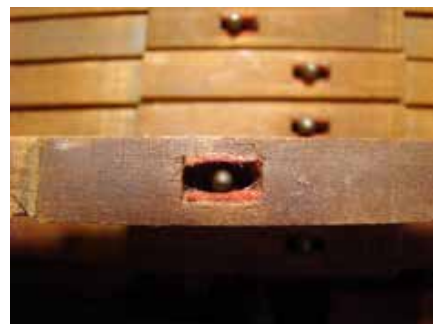
Photo 2: Carefully seat the key without smearing the glue.
