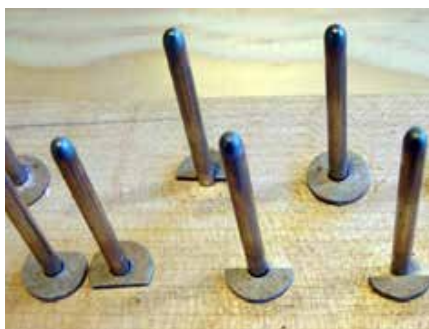
Photo 7: Cardboard punchings glued to the balance rail.
